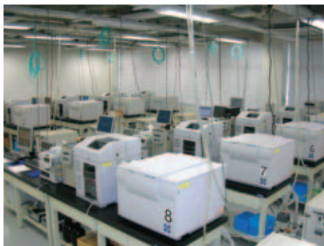
High-throughput and quantitative CE-MS methods which can measure thousands of charged metabolites. This is a powerful new research device developed by IAB.
