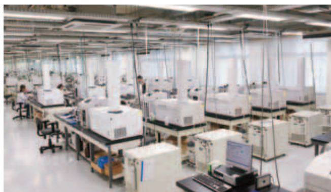
High-throughput and quantitative CE-MS methods that can measure thousands of charged intracellular metabolites. This is a powerful new device for metabolome research developed by IAB.
